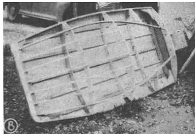
Showing bottom finished and deck framing in place.
