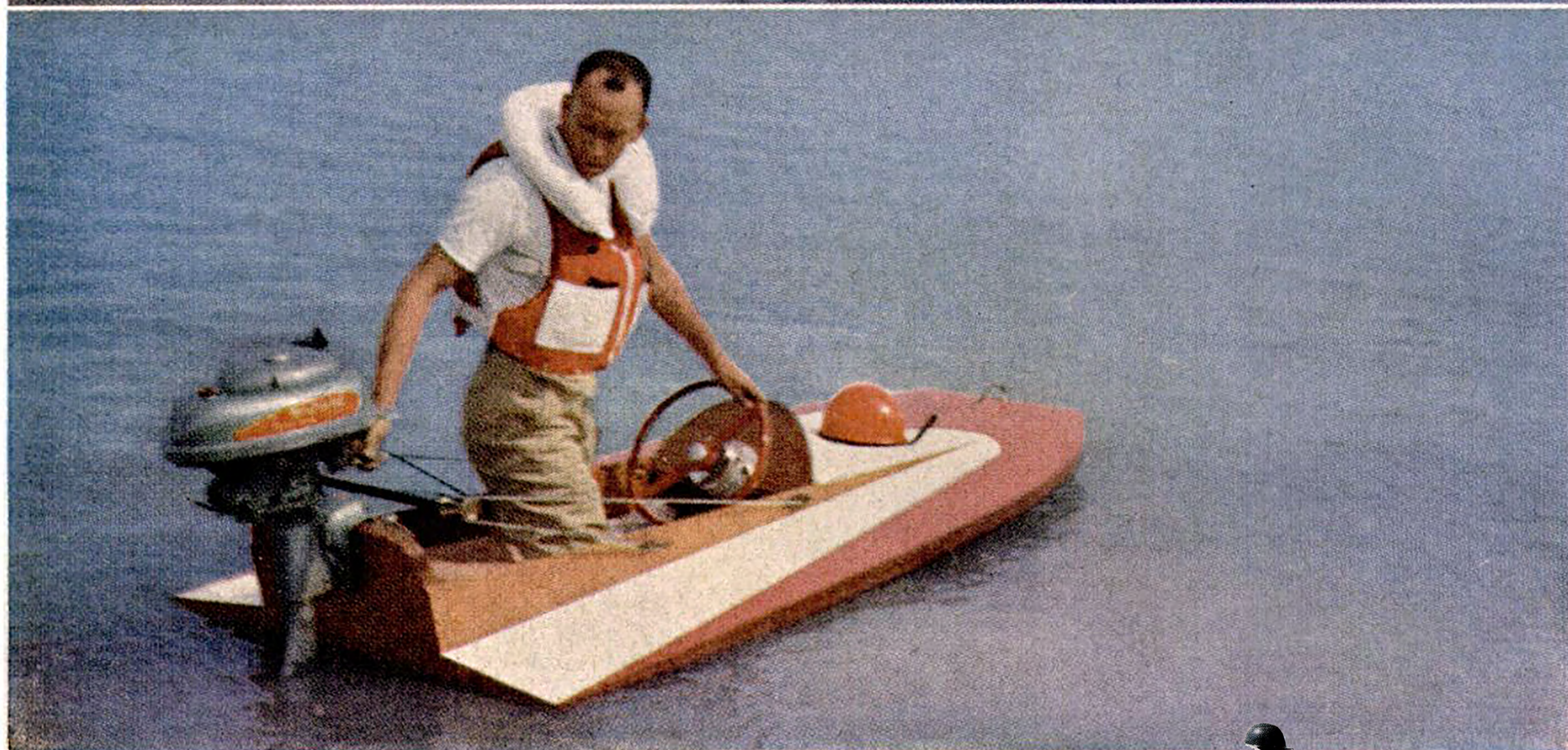
AN OLD HAND WITH HYDROS, Rogers says that this one likes motors in the 6-to-10-hp. range. His advice to novices: Get in some time at part throttle until you get the feel of the thing; avoid rough water or large wakes from other boats.
